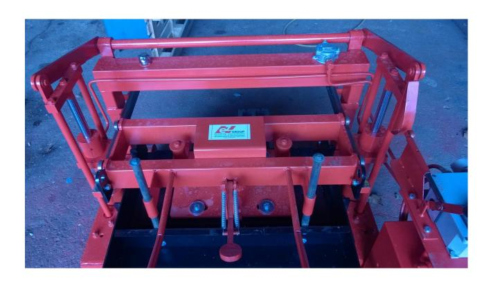
The laying M240 machine is specially designed for carrying blocks specially bricks and slabs of reinforced concrete measures varies with filling the hopper and ease of driving the production process
