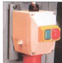
Magneto thermic switch
