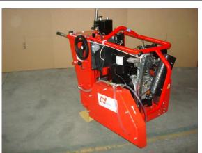
TS400 CONCRETE AND ASPHALT FLOOR SAW HONDA ENGINE
