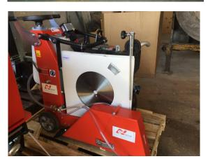
TS450 CONCRETE AND ASPHALT FLOOR SAW LOMBARDINI
