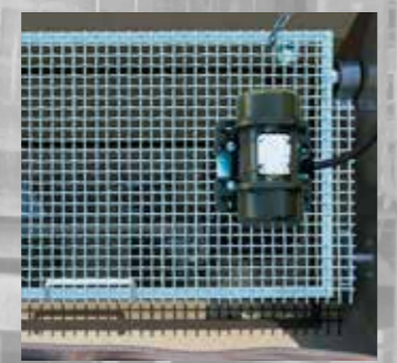
Vibrating grill with 15 mm mesh
